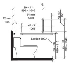
Three grab bars are required – 2 at the side wall and 1 at the back wall above the toilet.
