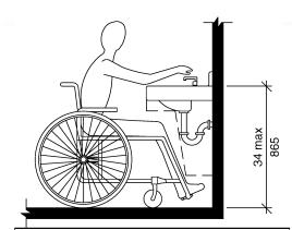
**606.6 Exposed Pipes and Surfaces.** Water supply and drainpipes under lavatories and sinks shall be insulated or otherwise configured to protect against contact. There shall be no sharp or abrasive surfaces under lavatories and sinks.
